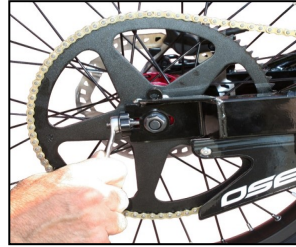
Chain tensioner nut 13mm
